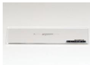
X-Y 校准标样 OLS50-CS-XY
